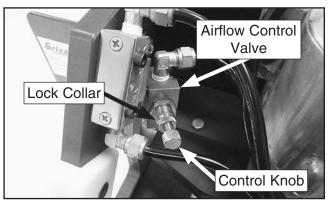
Figure 8. Airflow control valve.
